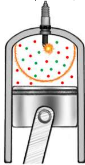
Spark ignition (Otto cycle) Gasoline, Methane, LPG
